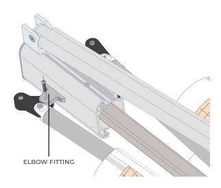
**STEP 3**REMOVE FLAT HEAD HEX SCREW FROM HEATER ARM AND BRACKET.
